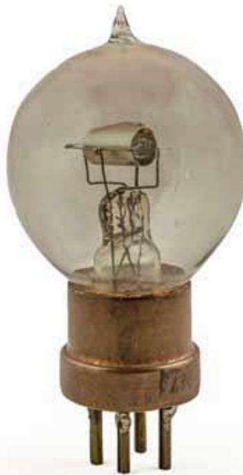
R-Type Thermionic Valve / Tube from around 1916 - 1920
