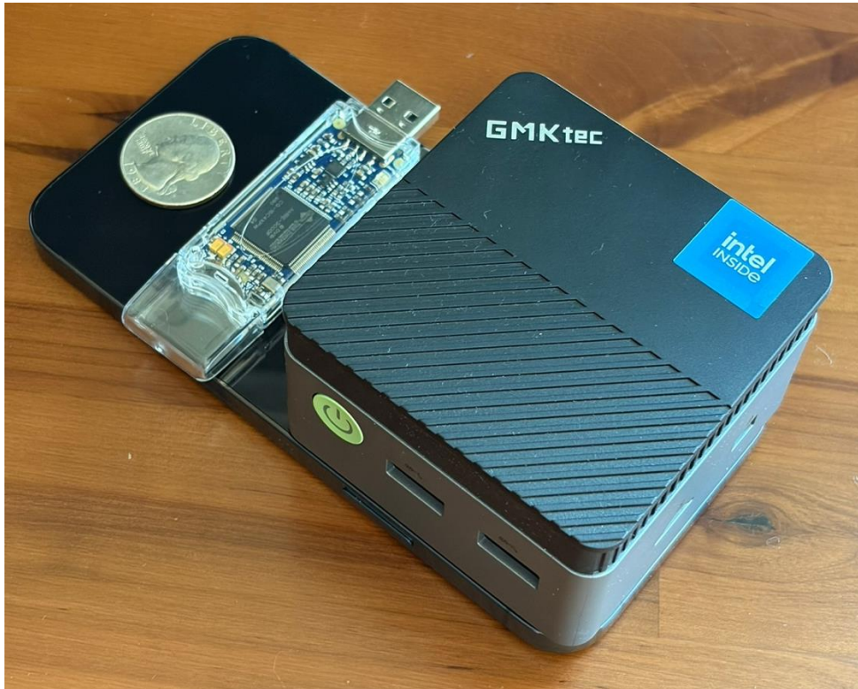
Figure 3. DVstick33 transcoder (left) and N95 mini-PC (right) placed on an iPhone 12 Pro for scale
