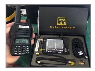
You can't see it due to the poor cell phone photography, but the Radio is transmitting on 145.51MHz the center frequency set on the Tiny SA. Yes I did ID for the test
