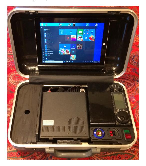
The Surface 3 fit nicely into the top cover of the Halliburton and is easily removable. I built a few wooden partitions in the case to separate the various pieces of equipment and to make compartments for the antennas, mic, key, and an HT. I added a SPDT center-off power switch which allows me to switch from internal power to external power, a digital voltmeter that includes a USB charging port and 2 Anderson power pole sockets for any external accessories.
