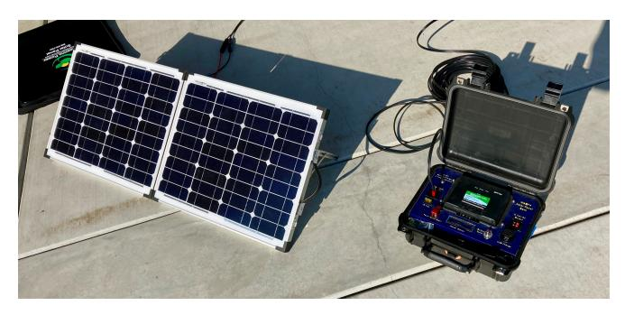
For PV panels I selected the Bioenno 60 Watt panel. This will recharge from depleted with about 4-5 hours of sun. The "power bank" powers my KX-3, pan adapter, USB SignaLink, Raspberry Pi and 10 inch monitor for a bit over 11 hours running digital modes 80% receive and 20% transmit and a bit over 8 hours with a 50%/50% receive/transmit. I've used it numerous times on trips and at Winter Field Day 2019, shown below.
