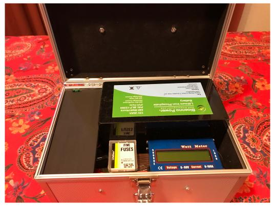
I bought an aluminum instrument case measuring 9" x 5" x 6". This was just large enough to house the battery, the inverter, and storage for an ammeter to measure current externally.
