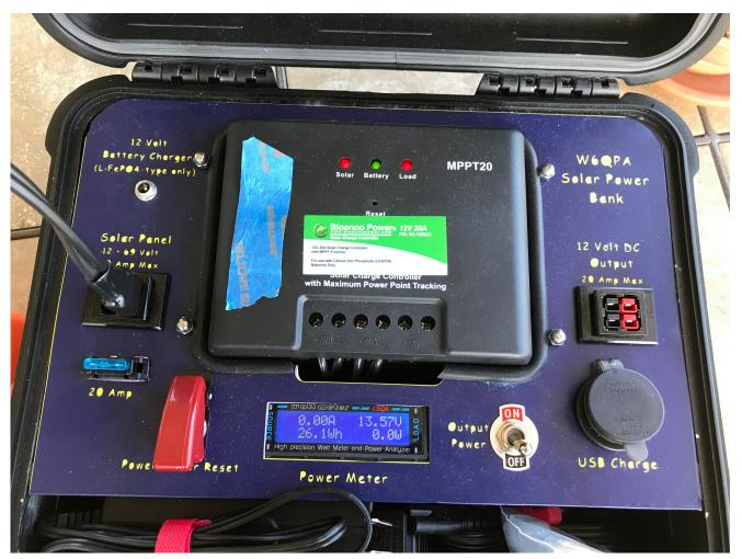
I selected the Bioenno 12 volt 12 Ah lithium iron phosphate (LiFePO4) battery. It is installed in a Harbor Freight "Apache" waterproof case, along with the charge controller, Anderson Power Pole connectors, a power meter and a USB charge port. If I were to do this again, I would use their smaller lighter charge controller, the MPPT controller is really only needed for multiple PV panel arrays.
