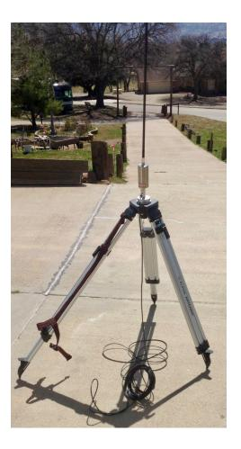
**Both antennas are easy to set up.** The Super Antenna is smaller and easier to store/transport, and I like the tuning coil so you can adjust to whatever band you are working. I suspect the Alpha antenna might perform better because it's taller. It definitely needs to be guyed because it is very top heavy, and will tip over with just a little breeze.
