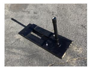
A few short pieces of I" x 4", I" x 6", a couple hinges, a short piece of pipe, a pipe flange, and some hardware will do the trick.
