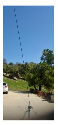
Super Antenna. The tripod is very sturdy and adjustable. The antenna collapses into several sections about 18-20" long. It comes with ground radials and also equipment to "Guy" the antenna down. It also comes with a 40' section of coax, which Alpha states must be used, or else the antenna will not work properly.
