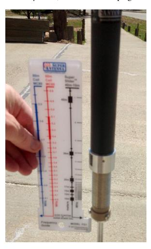
The tuning coil is adjusted by using the laminated card, and you slide it up/down to match the band you are working. I've only used it a few times and it works OK for short/medium distances. It would probably work better for someone who has more experience with HF than I do, and is willing to experiment with it.
