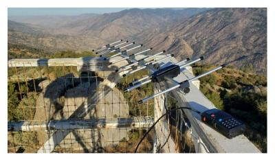
With a small directional antenna and 7 watts of power courtesy of an Anytone 868 Radio, I was able to hit the Hub of the Kern system up on Frazier at just under 90 miles away (though very scratchy) as well as the K6KGE, DMR repeater up at Shirley Peak. I wasn't prepared to communicate into, but I was also able to hear the cross-band repeater aboard the ISS on this same trip.
