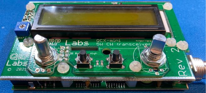
The small size is also achieved by redesigning what was once on a single PC board to three boards that are very tightly fit together. In this tiny package we still have a rig with with 200 Hz wide CW audio filter, receiver sensitivity of -117 dBm; thanks to Will, WA6LDQ for providing the test equipment and know how to run that test. It also has CAT control (emulates Kenwood TS-440 commands) built-in keyer, message memories and RIT/split support.
