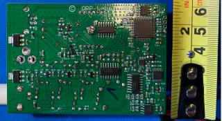
As in the QCX-mini, a lot of the circuitry is SMD components, factory installed. The bulk of the assembly on this one is winding ten toroids for the low-pass filters sections and a couple of transformers.
