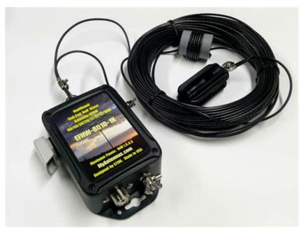
The EFHW-8010 is 130 feet long and works on 80/40/30/20/17/15/12/10m, while the EFHW-4010 is 63 feet long and works on 40/20/15/10m. They both will do Near Vertical Incidence Skywave (NVIS) on 40M or lower.
