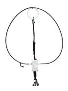
One of those in the first group is the Chameleon Antenna P-Loop portable mag loop antenna. Mine is the original version to which Chameleon has made some improvements. You have probably seen mag loop antennas made with tubes formed into a circle with a tuning box built into it (it's more complicated than that). This model is rather formed out of LRM-400 coax which you can detach and sort of roll into a more compact shape. They give you a mail carrier pouch to transport all the parts in.
