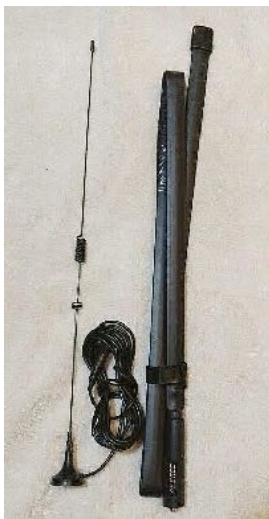
Mag mount (cookie sheet in duffel), 1 extra long Tactical antenna. Not shown, collapsible J-pole antenna, 1 Ground plane UHF antenna, (in car)
