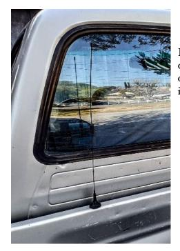
I used my old mag-mount attached to the back behind the driver side of the cab. The magnet on the mount is worthless over 5MPH so I taped it in place, then ran the antenna cable into the cab, under the seat and plugged into the radio.
