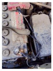
I installed a permanent power cable with an in-line fuse as well. I want the truck ready to go for the next time I need to go over rough ground.
