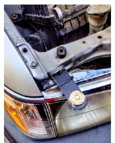
I fashioned an antenna mount from a hinge to mount the antenna above the right headlight.
