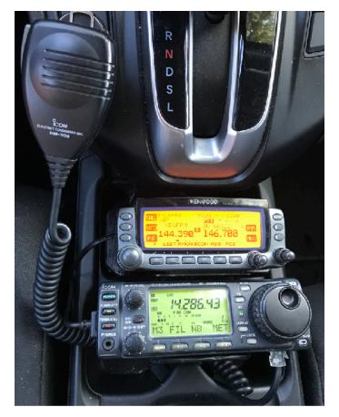
Both radios are operated with remote control heads mounted on the center console. I now have the capability to operate 75 meters through 440.
