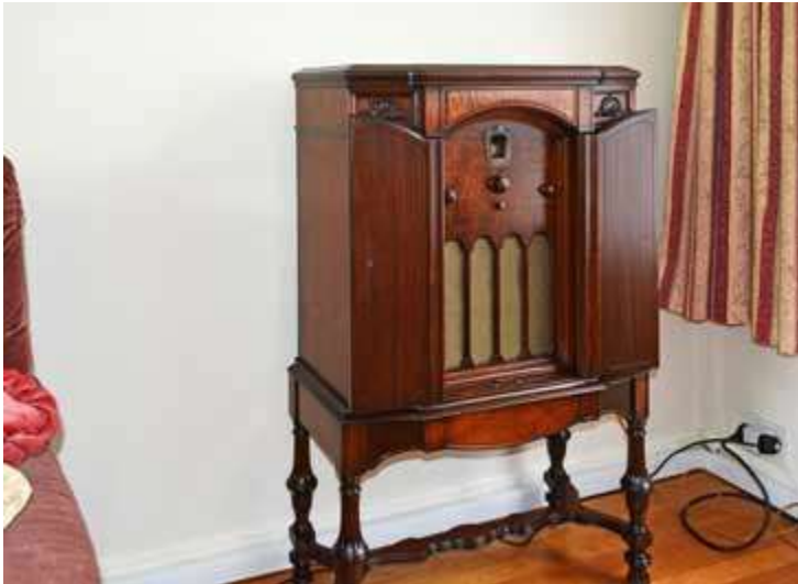
The 11 valve Philco 111 superhet from 1931
